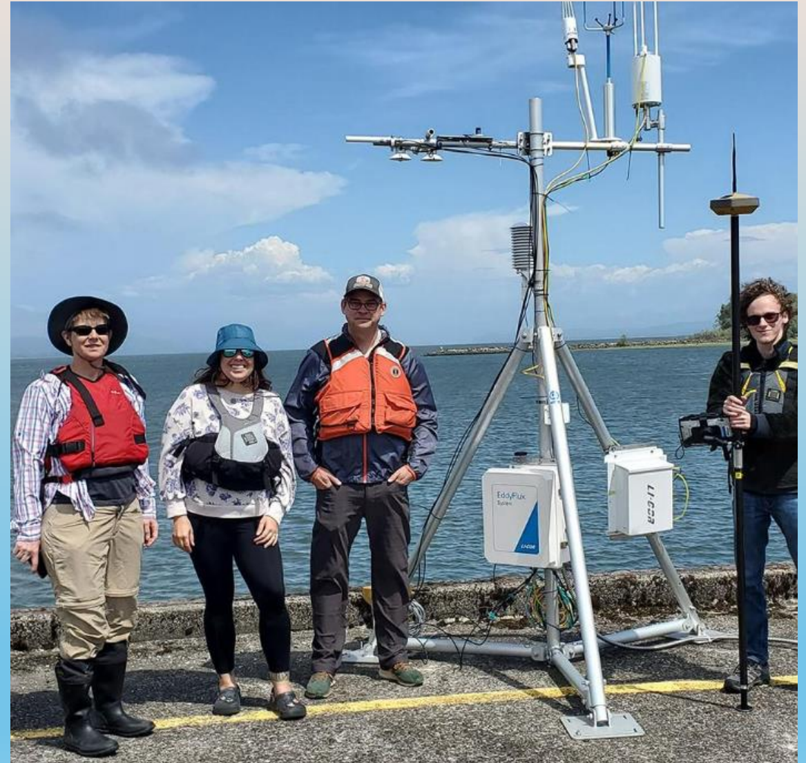
Researchers from OHSU, PSU and LCEP at Tongue Point, Astoria with one of the Eddy Covariance Flux towers
