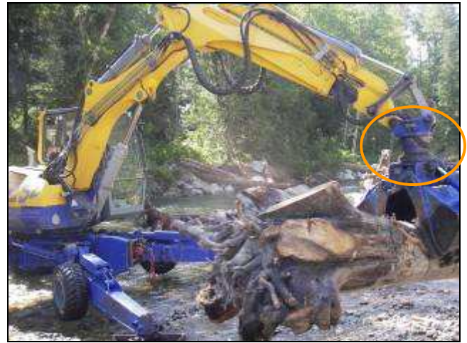
This “clam shell” style grapple/bucket has a swivelling head, allowing for greater manoeuvrability and precision with wood and rock placement.
