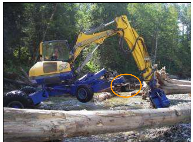
Flat pads on the front appendage prevents compression of the stream bed.
