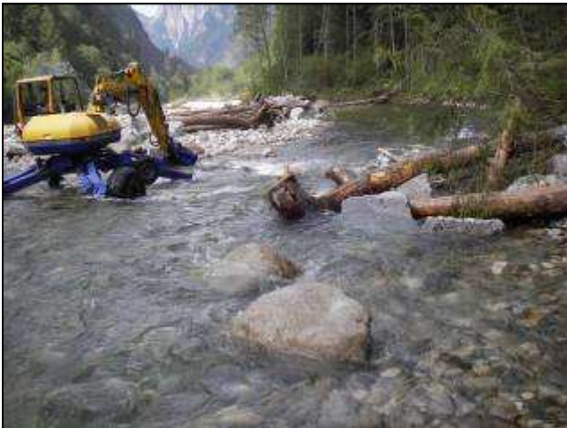
Balloon tires reduce compression of the stream bed.
