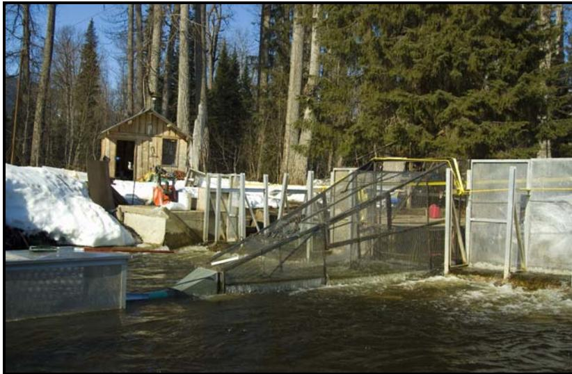
Figure 3. Smolt fyke trap in fishing position.
