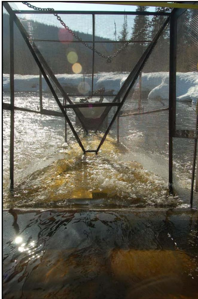
Figure 4. View upstream of the trap fykes under typical fishing conditions.
