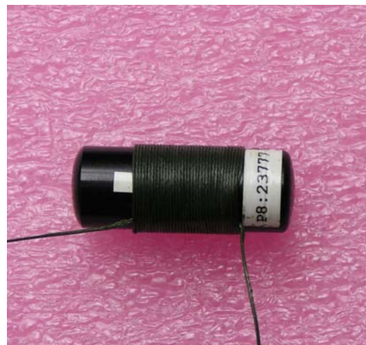
Figure 4. A Vemco V9-2H tag after attaching the spiderwire line as a harness.
