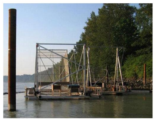
Figure 17. Photo of the Crescent site showing the position of the floating shoreline abutment, and both Crescent-Regular and Crescent-Large fishwheels, 6 August 2008.
