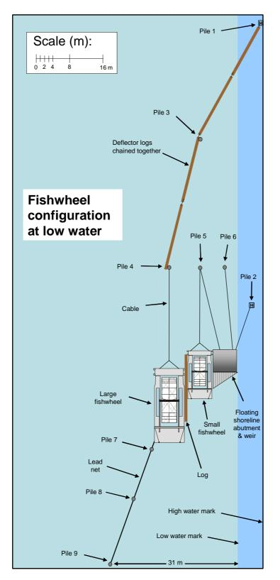
Figure 4. Schematic of the Crescent site showing the proposed locations for the pilings, fishwheels, floating shoreline abutment, deflector logs and barrier net.
