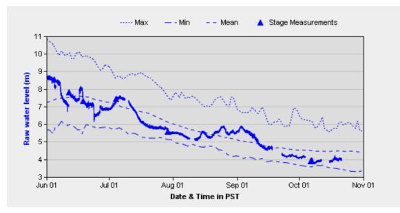
Figure 8. Fraser River water level (m) measured at the hydrometric station (08MF005) in Hope, BC from 1 June to 31 October 2008. Also shown are the historical mean, minimum, and maximum values (Environment Canada 2009).
