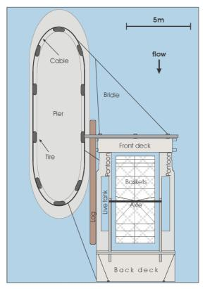
Figure 2. Schematic (top view) of a large, aluminum fishwheel attached to a concrete support pier at the Mission Railway Bridge on the Fraser River, 2008
