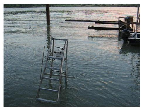
Figure 6. Photo showing DIDSON ladder mount positioned just off shore and downstream of the large fishwheel near Crescent Island.
