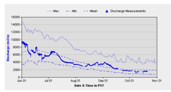
Figure 9. Fraser River discharge (m<sup>3</sup>·s<sup>-1</sup>) measured at the hydrometric station (08MF005) in Hope, BC from 1 June to 31 October 2008 (Environment Canada 2009). Also shown are the historical mean, minimum, and maximum values (Environment Canada 2009).
