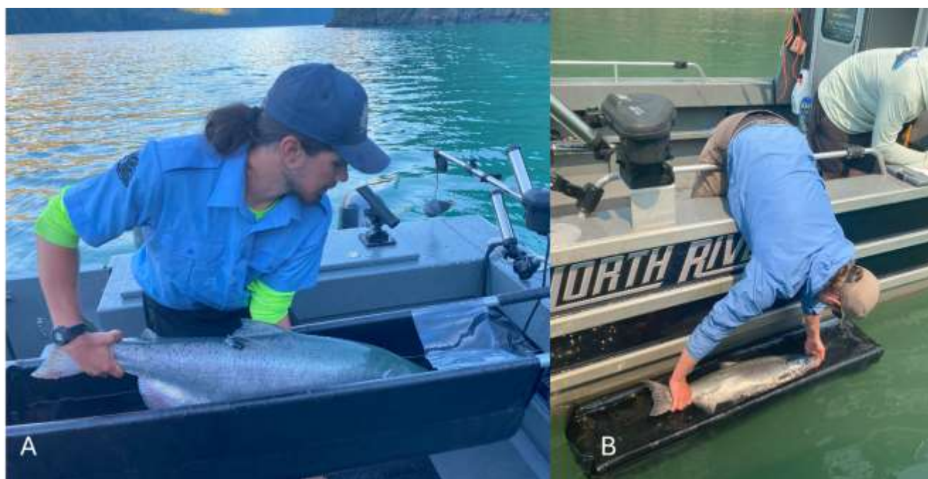
Figure 10. (A) On-boat sampling sling made from vinyl coated polyester developed for tagging and sampling live salmon with limited physical contact and impacts for the individual. (B) Modification of the sling with flotation that allowed fish to never be removed from the water but contained next to the vessel for tagging and sampling.
