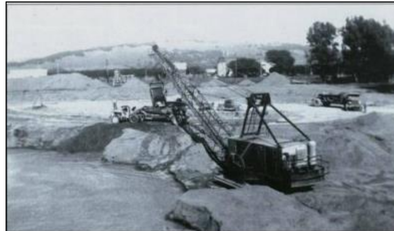
The shovel and horse-drawn wagon of the early days of gravel mining have been replaced by the high-extraction equipment in this c. 1940 picture. The production method, mining by drag line, involves swinging the bucket into the Russian River and dragging it ashore holding about three cubic yards of sand and gravel. The load is emptied into a waiting "cat wagon." (Courtesy of Rand Dericco.)
